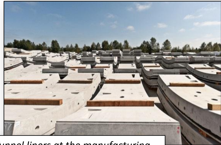
Tunnel liners at the manufacturing facility in Frederickson, Wash.
